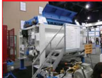
This Sicoma twin-shaft mixer has more arms than Doctor Octopus (24 vs. 6).
