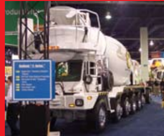
This seven-axle Oshkosh S-Series is a high-tech showcase with obstacle detection, rollover protection, composite drum, poly hopper and poly water tank.
