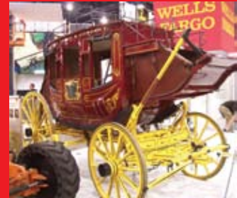
Abbot-Downing Concord Coach, built around 1870, was high-tech for its day with leather-sling suspension and bigger wheels than a rapper's Escalade.
