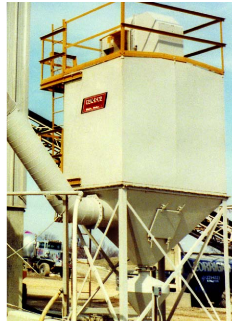
Ground-mounted dust control with automatic reclaim
